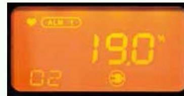
First alarm (orange)
